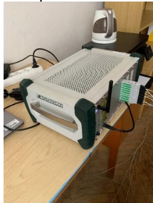
Figure 5: ALMEMO 500 device employed for recording temperature data
