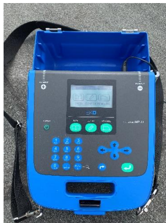
Figure 6: EKO MP-11 device employed to measure the electrical performance of photovoltaic modules
