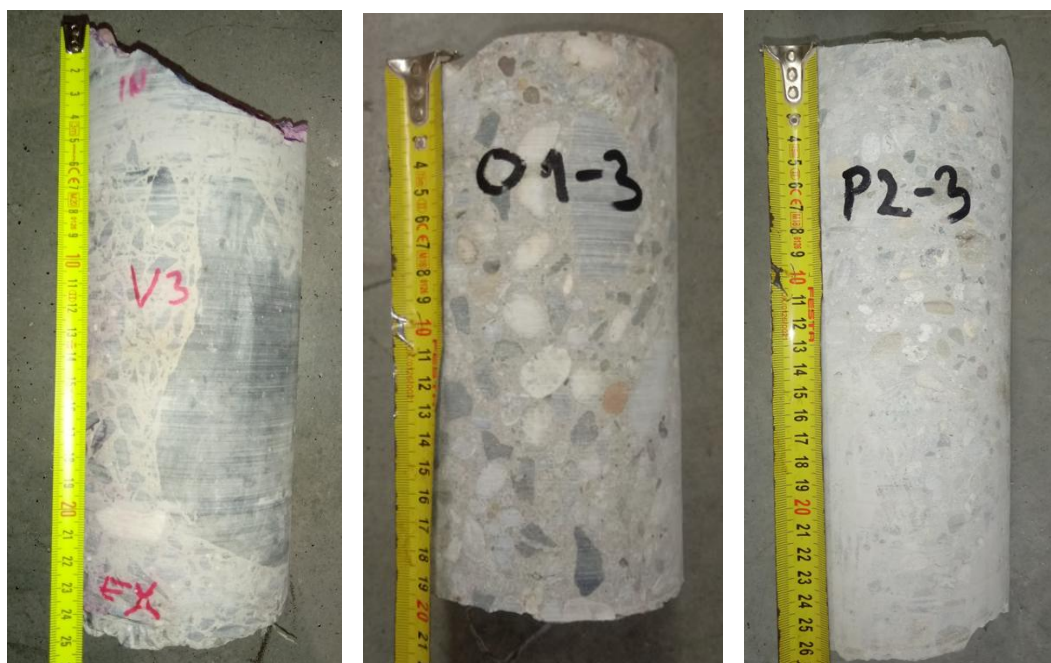
Figure 2: The Core drills with different aggregate sizes, from left: large, medium and small grains
