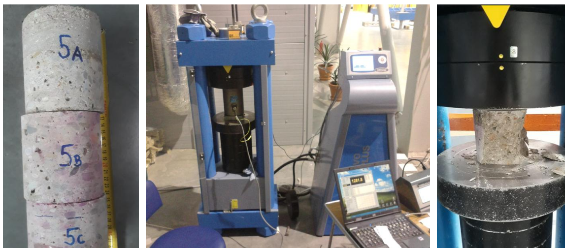
Figure 3: Left - prepared samples, middle - Matest press machine, right - damaged sample after testing
