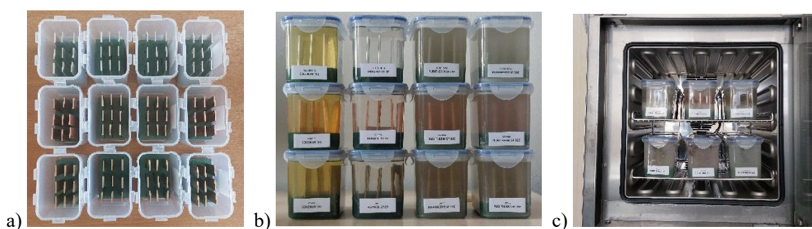
Figure 1: Preparation of samples for the PIT: a) prepared metallic samples before immersion; b) metallic samples immersed in PCM in sealed containers; c) placement of samples in the environmental chamber
