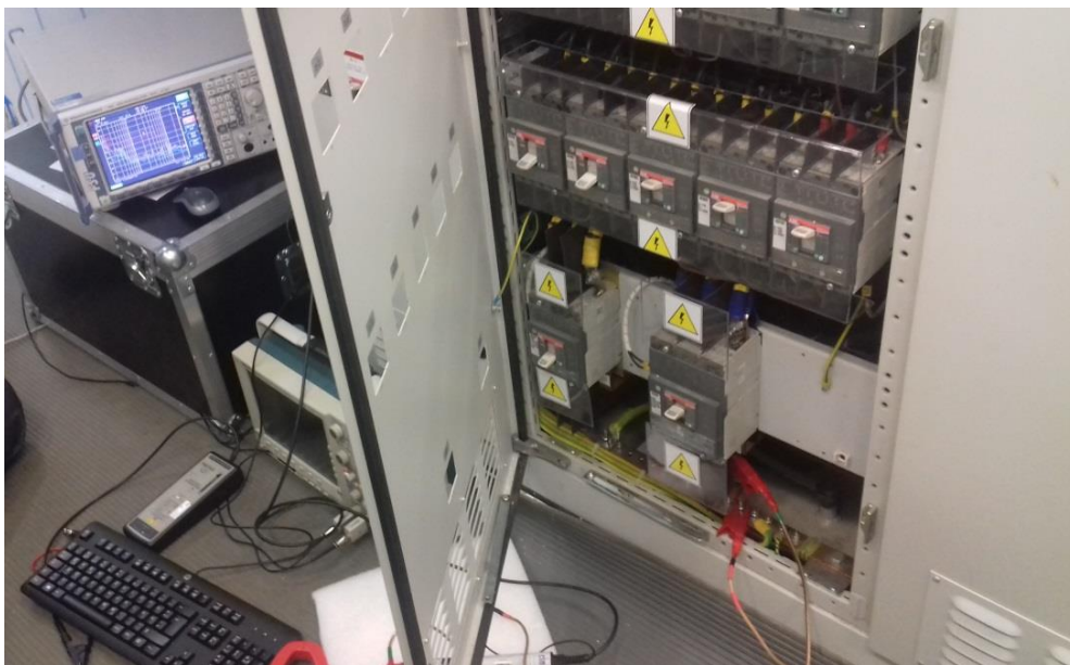
Fig. 3. Test set-up for free standing EUT, in situ test
