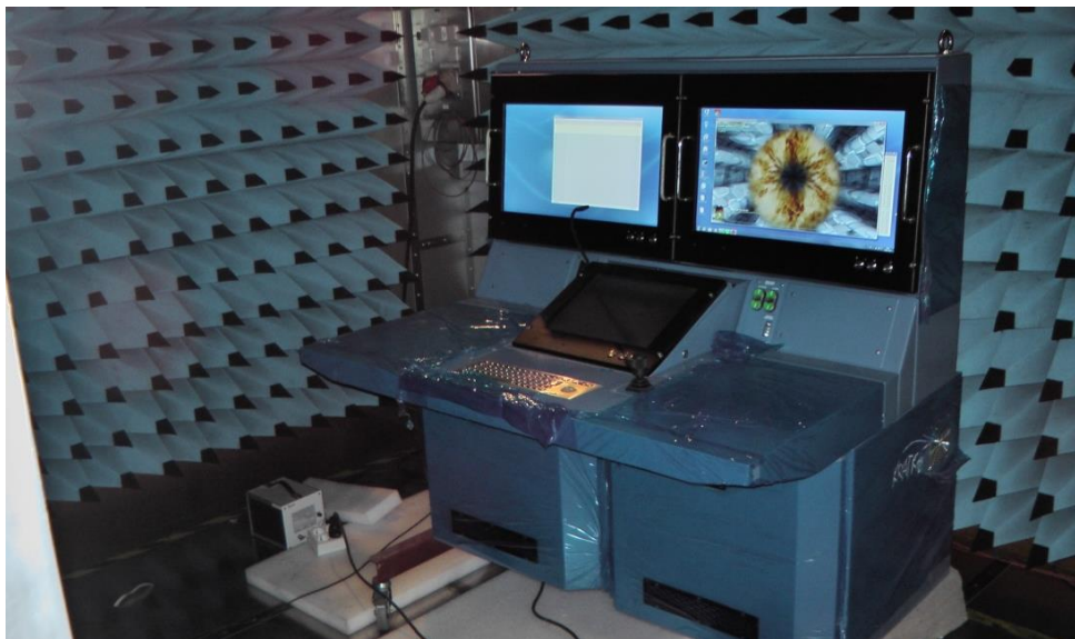
Fig. 6. Test set-up for free standing EUT in shielded enclosure according
