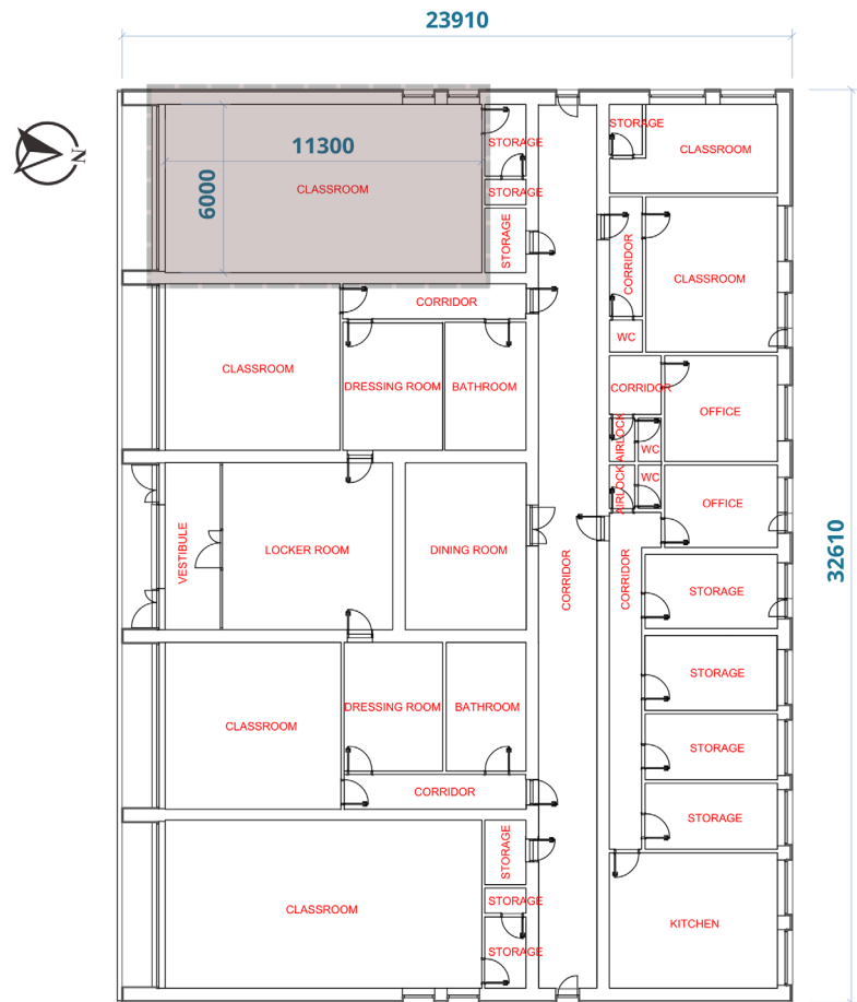
Fig. 2 Floor plan of the kindergarten building in Miloslavov with the location and basic dimensions of the corner classroom analysed
