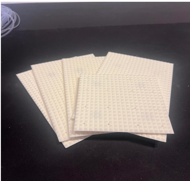
Fig. 6 Types of geometric wall roughness.
