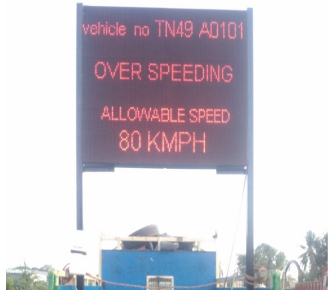
Fig. 9 The VMS's number plate display for a speeding vehicle
