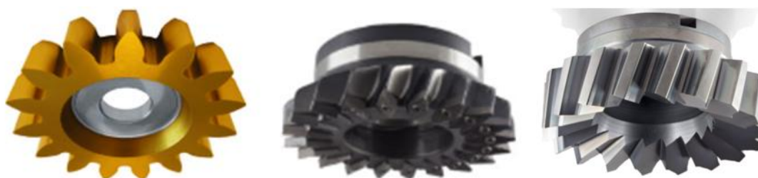
Fig.12 Solid skiving cutters with a zero rake angle
