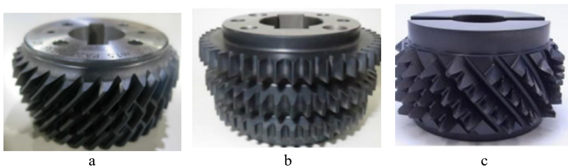
Fig.13 Conical skiving cutters with helical teeth (a) and straight teeth (b) and spur cutter (c)[20]
