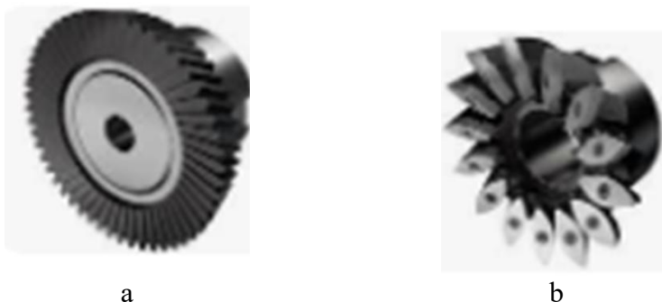
Fig. 9 Solid cutter (a) and cutter with inserts (b)
