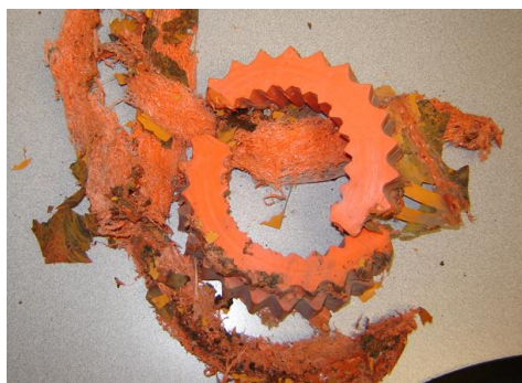
Fig. 1 Photo of destroyed elastic spider coupling element [1]
