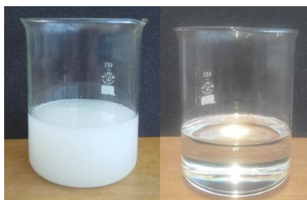
Fig. 1 Water contaminated resin (left) and pure epoxy resin (right)
