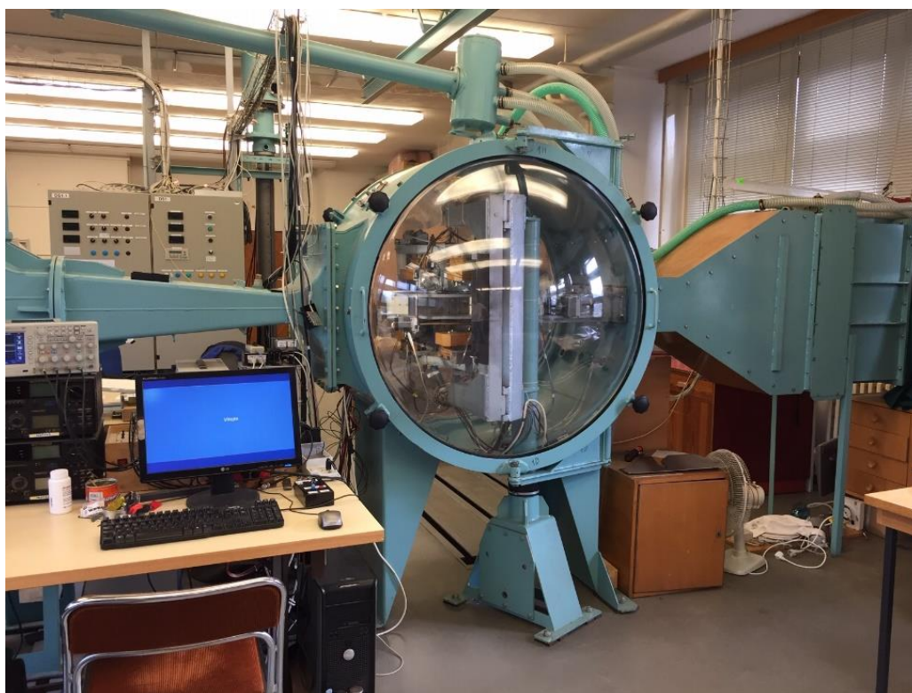
Fig. 1. Vacuum drum chamber with a test section: the air flow direction is from right to left
