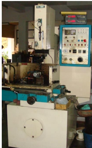
Fig. 2.1 Electronica Die sinking Commercial microEDM Machining Setup
