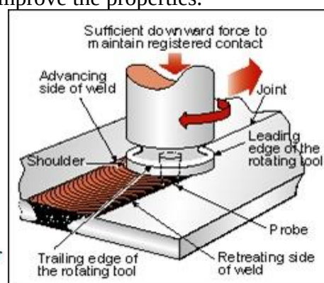
Fig. 2 (Schematic diagram of FS process)
