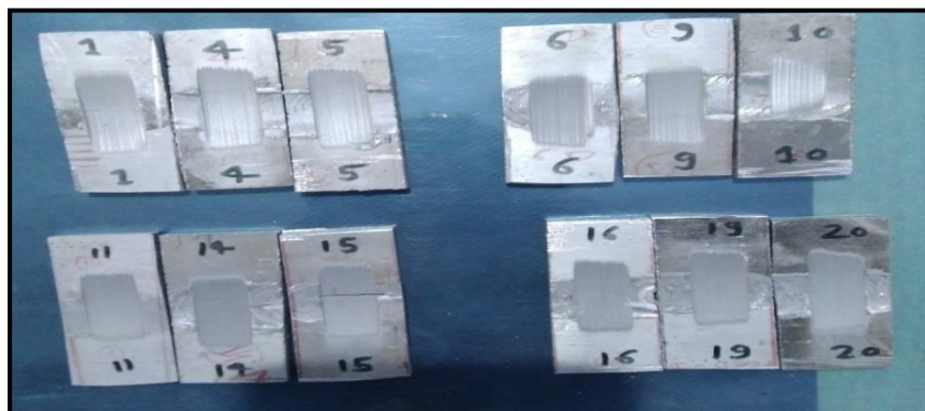
Fig. 4 FSW samples after sand abrasion test
