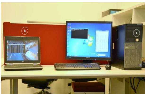
Figure 4. Unmodified USB device (memory stick) (A) transmits information to a nearby receiver (B) via electromagnetic waves emitted by the bus [29].
