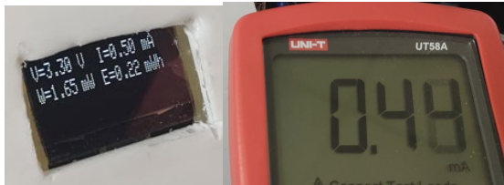
Figure 22. Comparison of the current result provided by the system with the one provided by the ammeter.
