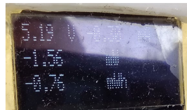
Figure 15. The voltage displayed by the system when it is cloudy.
