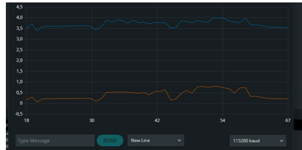
Figure 24. Data acquisition for current and voltage in Arduino IDE – Case 1.
