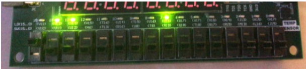
Figure 19. SLC results using the Nexys4DDR platform – Case 2 – CK=1, Q_0Q_1Q_2=011 .
