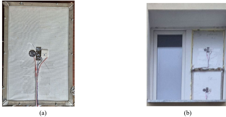
Fig. 1. Vacuum insulation panels: (a) used in experimental study with installed heat flux density and temperature sensors; (b) mounted in a window frame for field testing.
