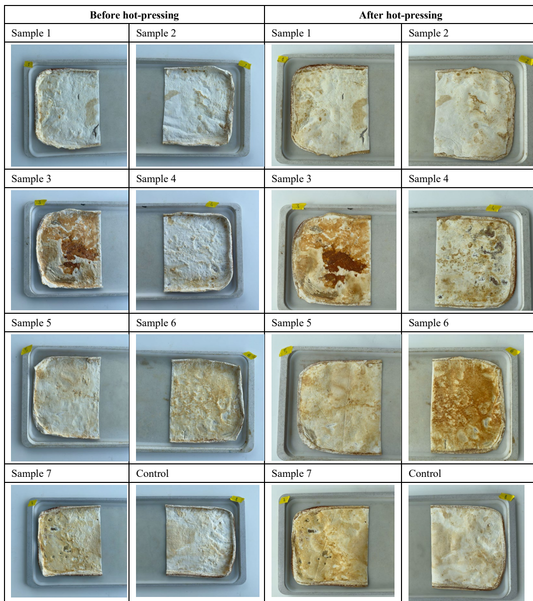
Fig. 5. Images of the T. versicolor -based mycelium mats before (left) and after (right) hot pressing at 100 °C for 1 minute. All mats received additional surface coating except for the control mats.
