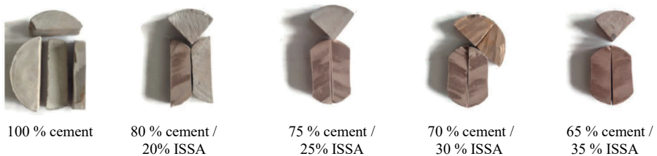
Fig. 1. Hardened cement blocks with varying proportions of incineration sewage sludge ash (ISSA).
