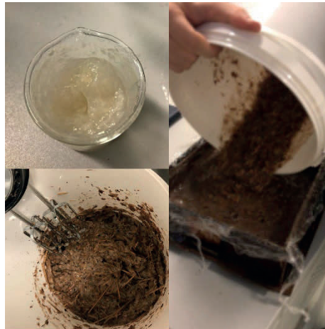
Fig. 2. Mixing mycelial material.
