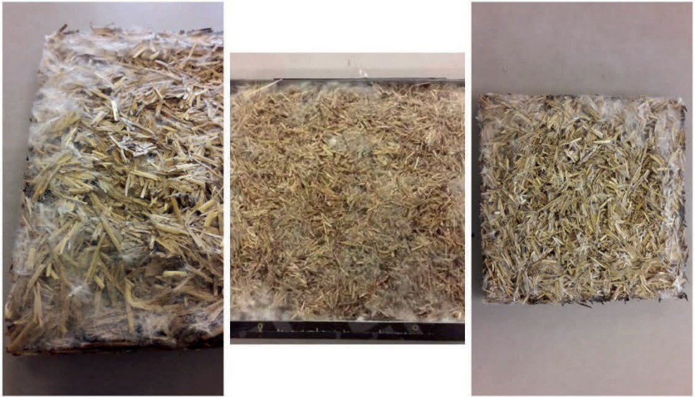
Fig. 3. Mycelium material after drying.
