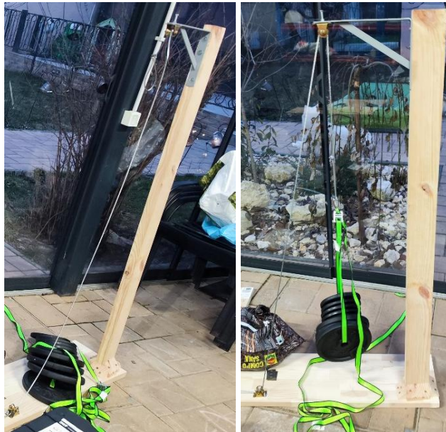
Figure 16. Installed stilps and anchorage on the wooden base plate
