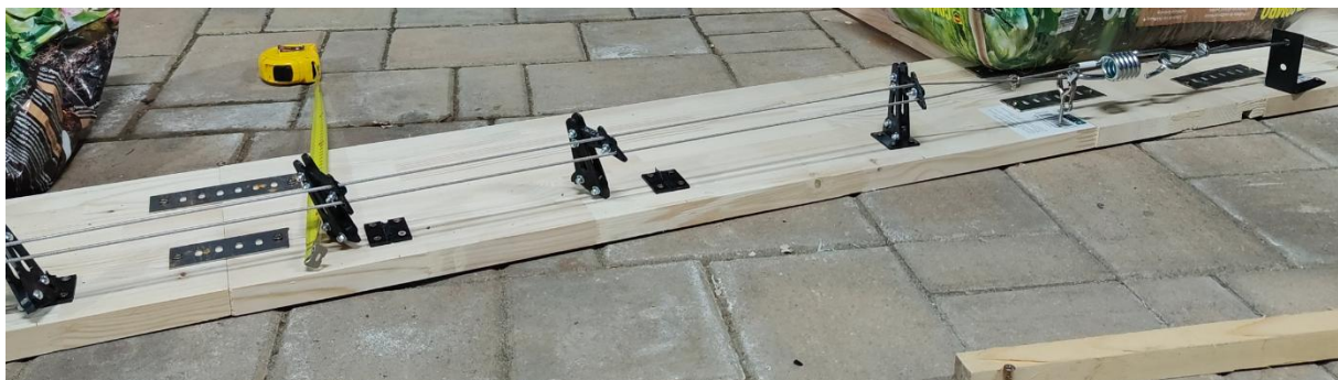
Figure 19. Scaled guardrail after crash test
