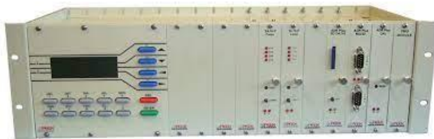
Figure 1. ADR 3000 – WIM system (Weight in Motion)
