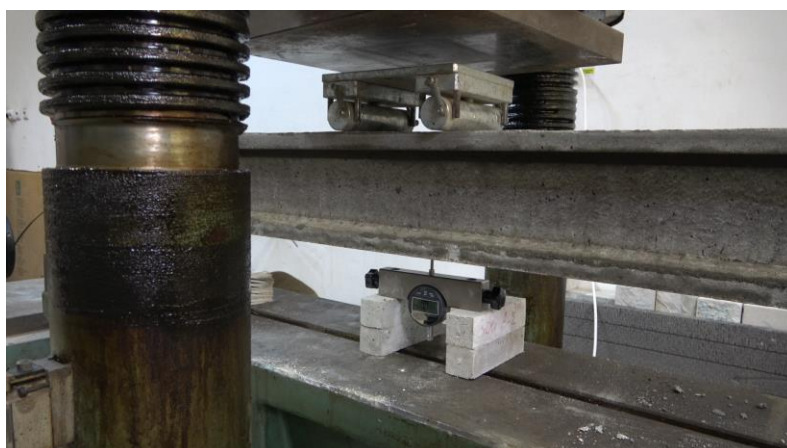
Figure 16. Flexural load test
