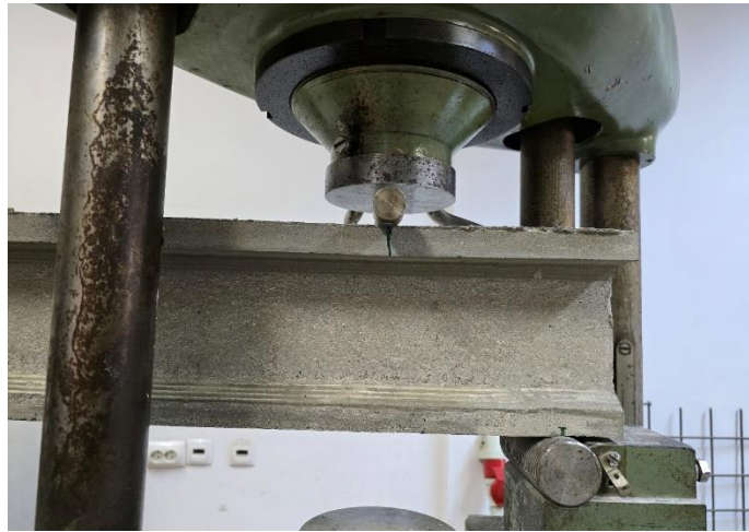
Figure 17. Shear load test
