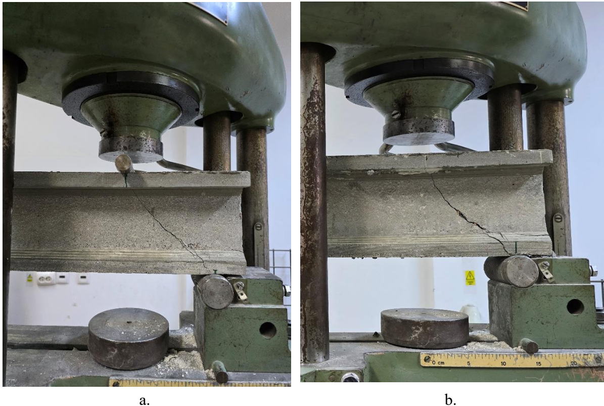
Figure 20. Comparison of shear failure mode: a. steel reinforcement; b. GFRP reinforcement
