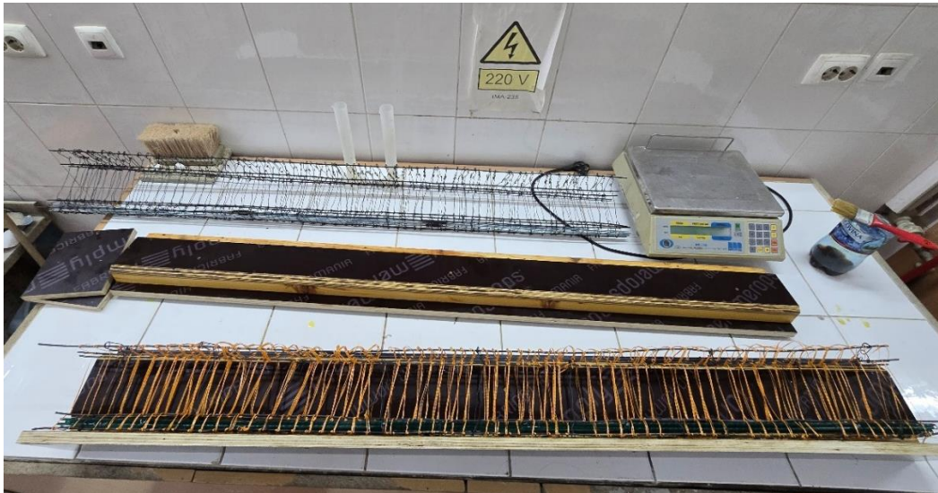
Figure 14. Details of reinforcement cage fabrication and placement in the formwork
