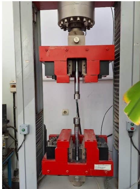
Figure 9. Tensile testing of reinforcement bars
