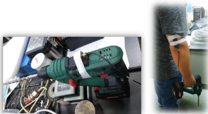
Figure 3. Sensor attached to the drill and the operator's elbow [1] (images from the author's personal archive)
