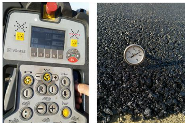
a) The finisher thermometer b) Manual thermometer
