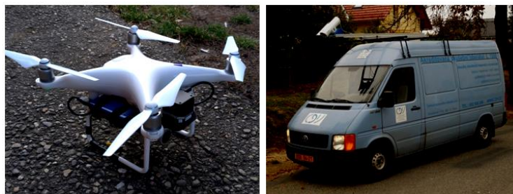
a) Thermal camera mounted aboard an UAV b) Thermal camera mounted on a land vehicle [5]
