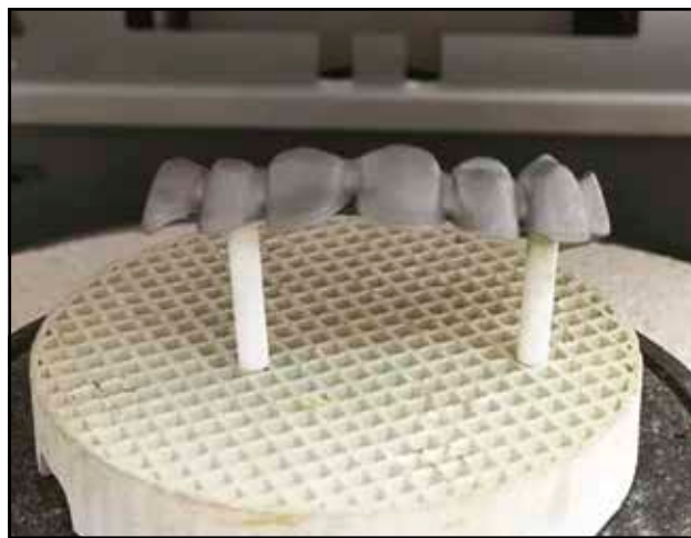
Figure 8. The metal substructure at the beginning of the oxidation program using the firing furnace.
