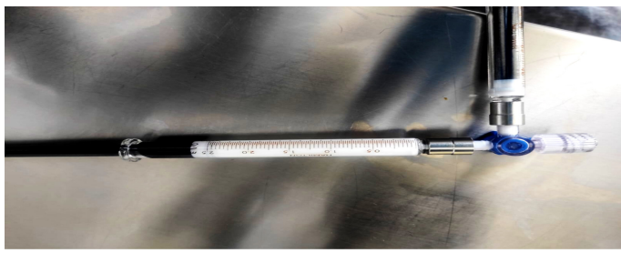
Figure 1 - Attaching the 2.5 mL Hamilton® syringes to the two-way stopcock with Luer-Lock to prepare the emulsion.
