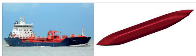
Fig. 3. MT Uikku and the finite element model used in the simulations
