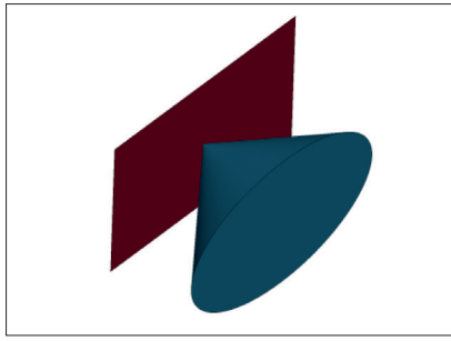
Fig. 4. Finite element model of a steel plate impacting on conical sea ice
