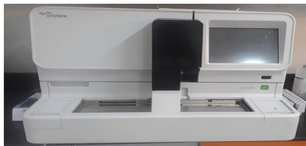
Figure 1. CS-1600, automated hemostasis analyzer (Sysmex, Wakinohama, Japan).
