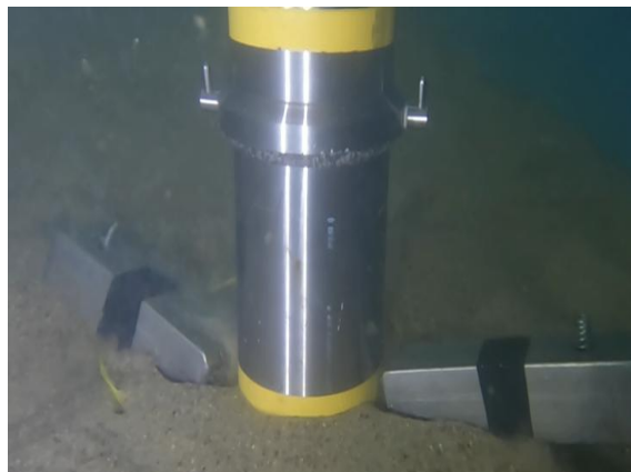
Fig. 7 Release of ballast during Test No. 3.
