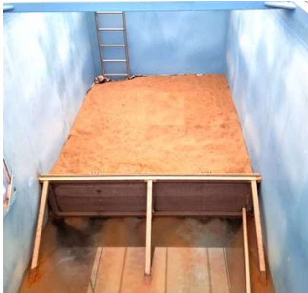
Fig. 1 Simulating sandy seabed conditions in a test pool during testing.
