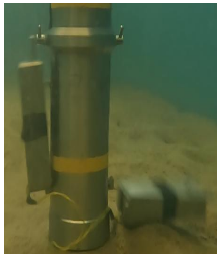
Fig. 3 Release of ballast during Test No. 1.
