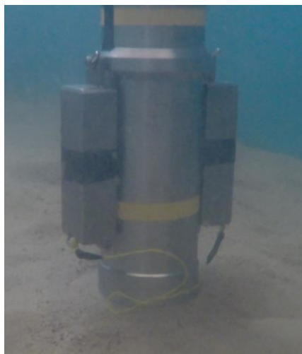
Fig. 2 Float with the rescue device resting on the test bottom in the pool.
