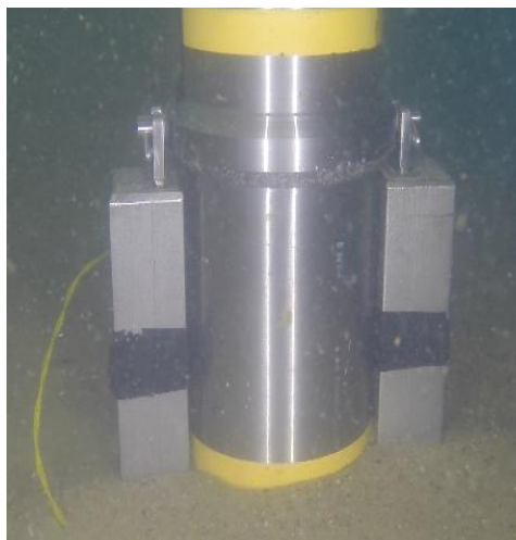
Fig. 6 Float with the rescue device embedded in the bottom to a depth of approx. 10 cm.
