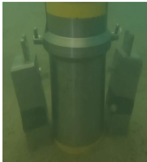
Fig. 9 Release of ballast during Test No. 4.
