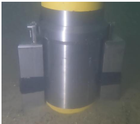
Fig. 8 Float with the rescue device embedded in the bottom to a depth of approx. 10 cm – Test No. 4.
