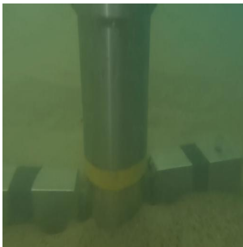
Fig. 10 Test No. 4 Float in a horizontal position before releasing the float.
