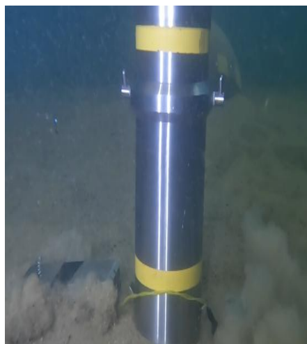
Fig. 5 Release of ballast during Test No. 2.
