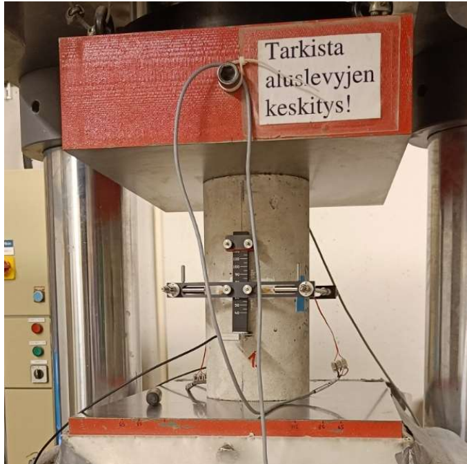
Figure 2 – Test setup of a 150 × 300 mm concrete cylinder for measuring elastic modulus and Poisson's ratio under compression from the ELC (elastic properties and carbonation) group
