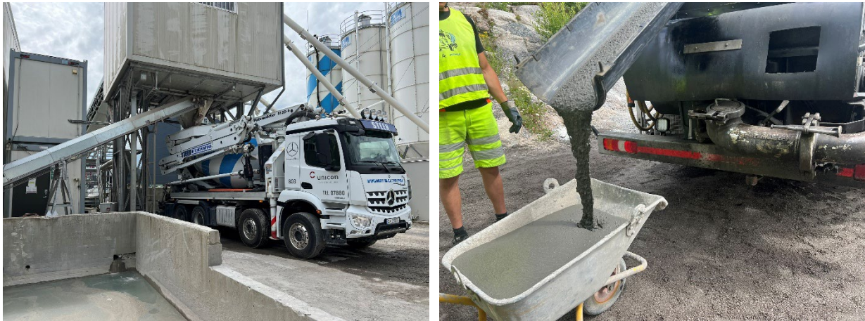
Figure 4 – Production of UHPFRC at Norwegian RMC plant.
