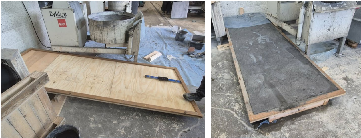
Figure 2 – Suitability test for inclined slab.
