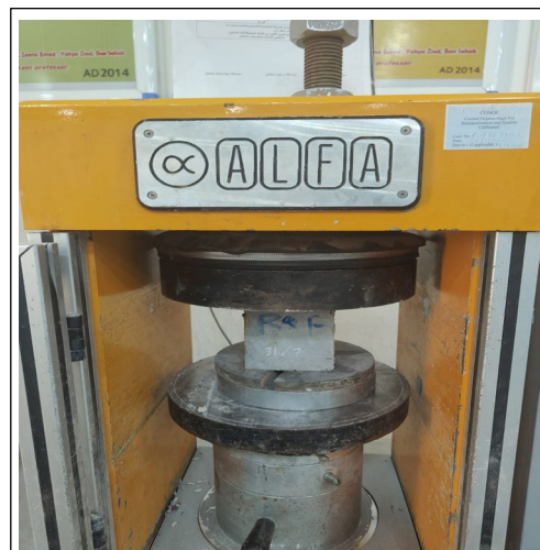
Figure 3 – Compressive Strength Test
