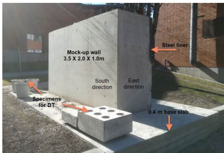
Figure 6 – Mock-up wall on its foundation [14].
