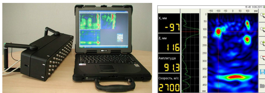
Figure 5 – Example of a UPE system, array of transducers and measurement images [12].
