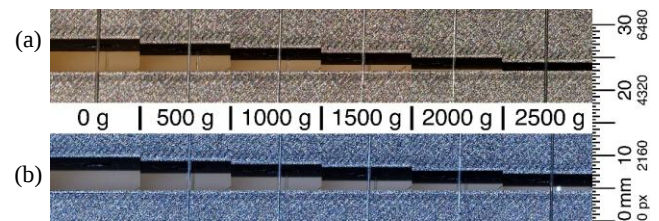
Fig. 12. Optical measurement of the dependence of the distance between plates G on the magnitude of the force acting on CCCMB (without conductive plates): (a) center-supported measurement; (b) edge-supported measurement.
