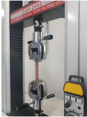
Fig. 6 Tensile Testing of Gnetum Gnemom L. Woven
