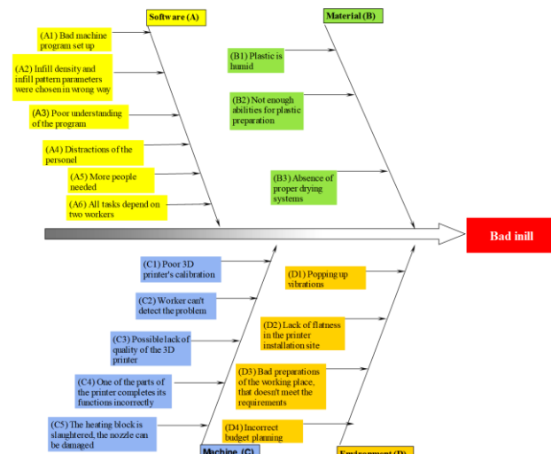
Fig. 1 Ishikawa Diagram for the first defect – Bad infill
