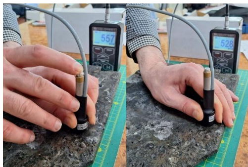
Fig. 8 The hardness measurement procedure test results for hardfaced Armox® 440T steel armor plates after ballistic tests
