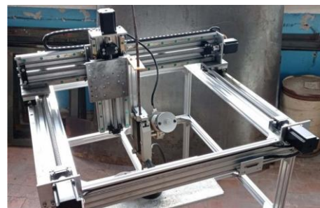
Fig. 2 Laboratory automated FCAW machine
