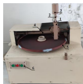
Fig. 1 Used testing equipment, where: 1 – Sample holder head, 2 – Sample holder, 3 – Weights, 4 – Feed mechanism, 5 – Rotating disc with bonded abrasive, 6 – Control unit
