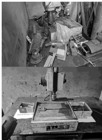
Fig. 3 Drilling station before and after the implementation of 5S methodology
