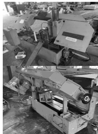
Fig. 4 Band saw station before and after the implementation of 5S methodology
