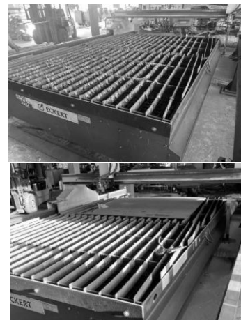
Fig. 1 Plasma cutting station before and after implementation of 5S methodology
