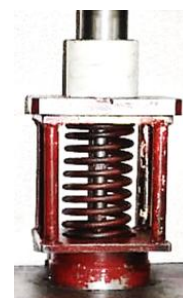
Fig 8 Shows The Deep Drawing die Utilized
