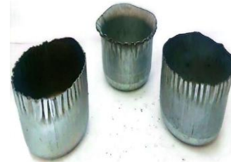
Fig. 14 The rim of the cup is in a state of destruction
