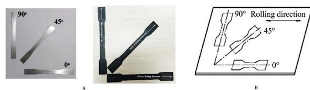
Fig. 3 (A) Specimens angle after cutting, (B) Desing of Sheet Metal
