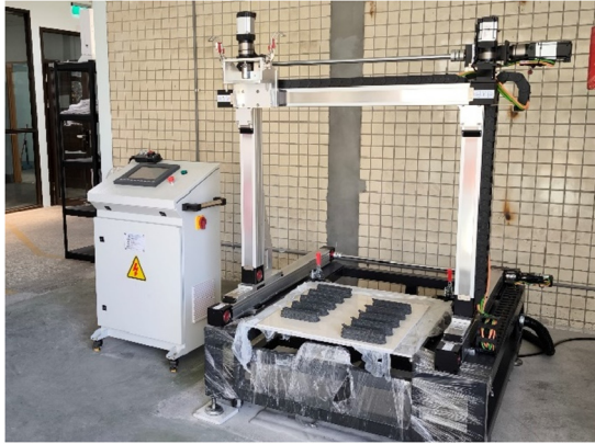
Figure 4. Appearance of the mortar-type 3D printer.
