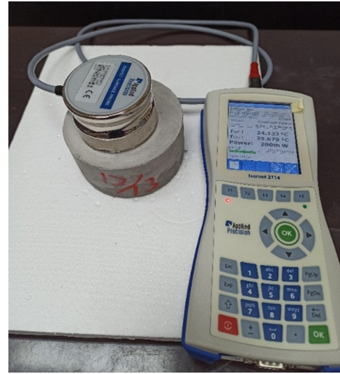
Figure 6. Appearance of the thermal conductivity device.
