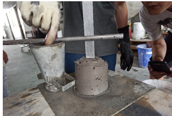
Figure 3. Appearance of the mini-slump test.
