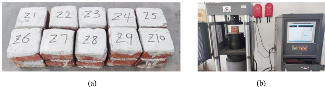
Figure 7. Compressive strength test of a single brick. (a) Brick specimens. (b) Testing apparatus.
