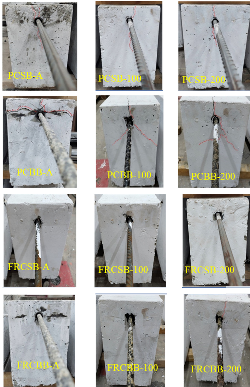
Figure 5. Failure modes of rebars embedded in PC and FRC.
