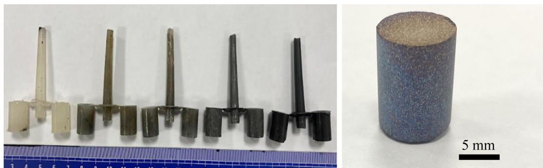
Figure 3. Photograph of injected specimens with varied metal contents (left), photograph of sintered specimen (right).
