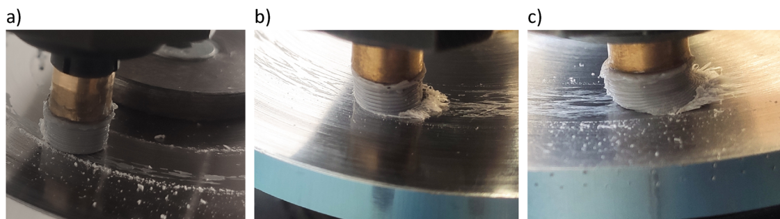
Figure 4. PLA specimen after interaction with a steel disc at parameters: (a) v = 1 m/s and p = 0.05 MPa, visible scattered loose wear products; (b) v = 1 m/s and p = 0.1 MPa, visible “braid, plume” behind the specimen, and “shreds” of plastic on the disc; and (c) v = 1 m/s and p = 0.4 MPa, specimen deformed from temperature.
