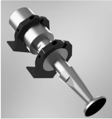
Figure 7. View of 3D model of the ultrasonic system with the working plate for ultrasonic wave concentration.
