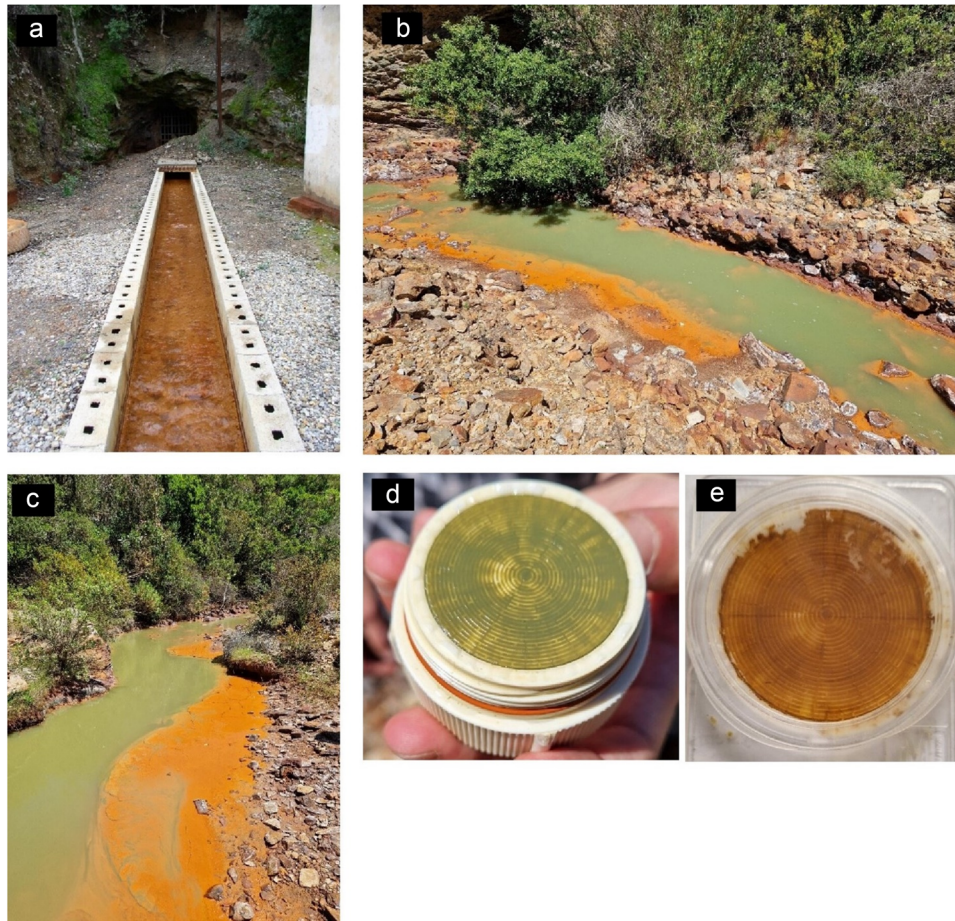
Figure 2. (a) Water outlet from the Casargiu mining gallery (CAS1); (b and c) the RIV3 sampling site in the Rio Irvi where “green rust” formation is evident; (d) “Green rust” on 0.45- \mu\text{m} filter collected filtering water from the Rio Irvi at the RIV3 sampling site; (e) same filter as d after 24 h where the colour change is due to oxidation of Fe(II), present in the composition of the “green rust”, to Fe(III).
