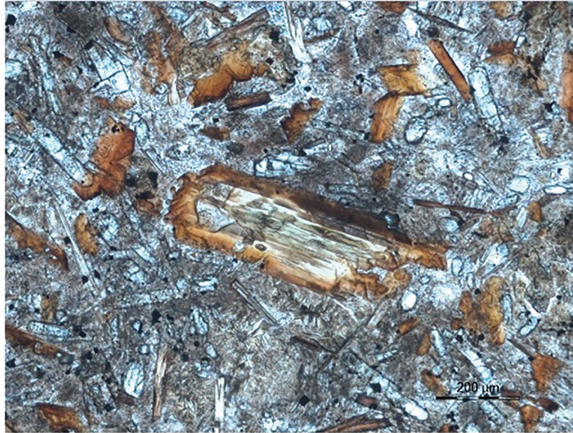
Figure 3. A photomicrograph with phlogopite microphenocrysts in PPL from the Limnos island para-lamproite sample GL28. The rock also contains phenocrysts of serpentinized forsteritic olivine and diopside, and magnesiochromite grains in a groundmass which additionally includes sanidine.
